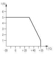
Continuous current limit curve (Current over 2 contacts) M8367
