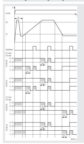
P1max/P2max: Overload monitoring with prewarning P1min/P2max: Under- and overload monitoring
