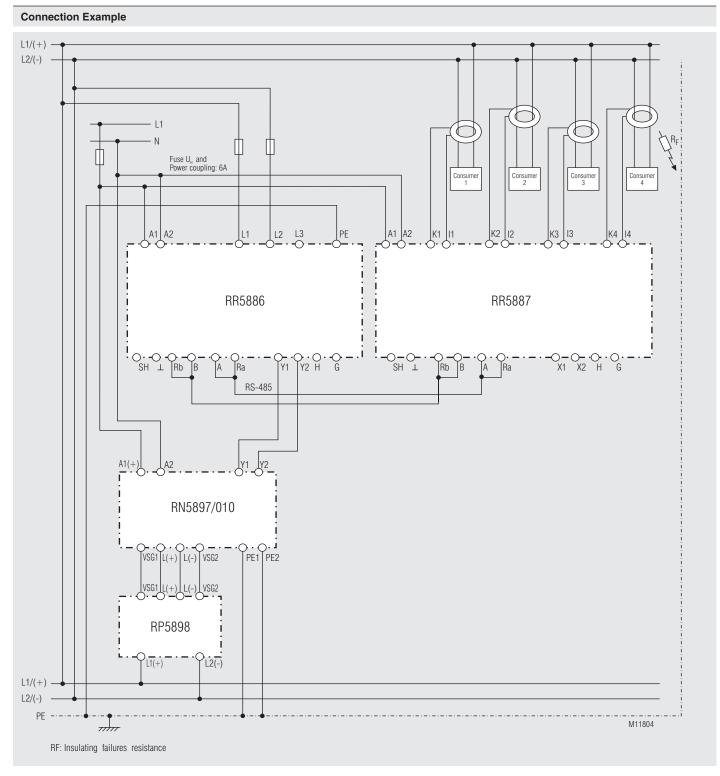
Insulation monitoring and insulation fault detection with 4 connected current transformers in a DC/AC network with subdistribution - insulation fault detection can be controlled by the insulation monitor (RN 5897/010); bus termination of the first and last device on the RS-485 bus.
