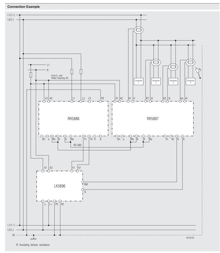
Insulation monitoring and insulation fault detection with 4 connected current transformers in a AC (DC) - network with subdistribution - insulation fault detection can be controlled by the insulation monitor /LK 5896); bus termination of the first and last device on the RS-485 bus.
