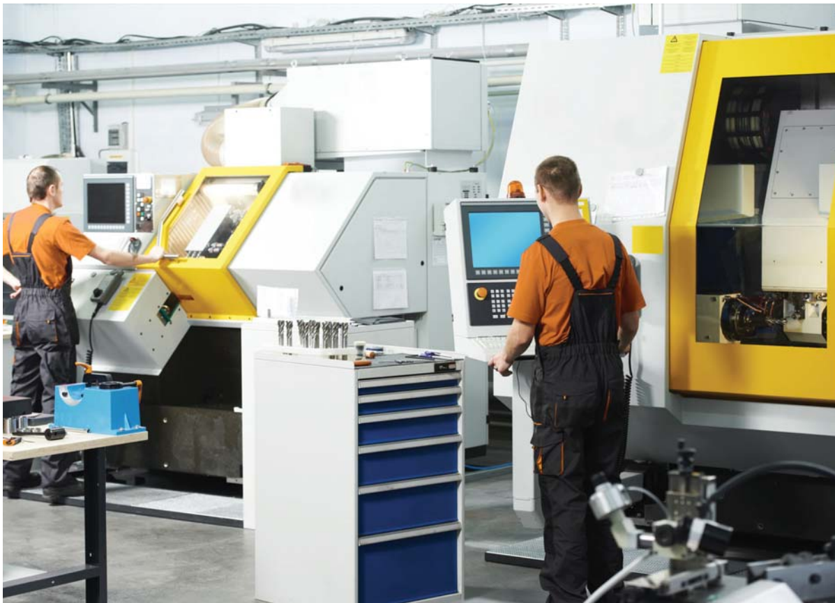
Persons must be safely protected from moving machine parts. It must only be possible to open safety doors when there is no longer any danger.
