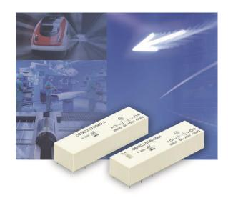
Reduced energy consumption in the relay's design was also a major focus. This is how this energy-saver only requires brief switching pulses of a few milliseconds to put their contacts into a defined switch position. Both magnetic systems make do with 1.2W for the interlock device and 0.7 W for the release device. This also makes the relay ideal for applications with high packing densities in thermally-sensitive environments.
