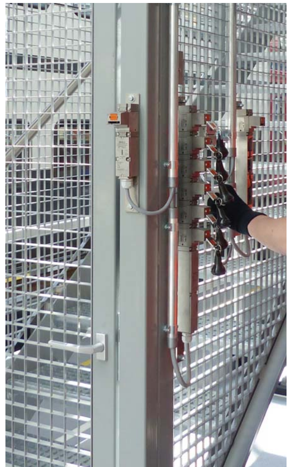
Electromechanical safety door protection with release of 6 keys for the opening of wirelessly safeguarded side doors
