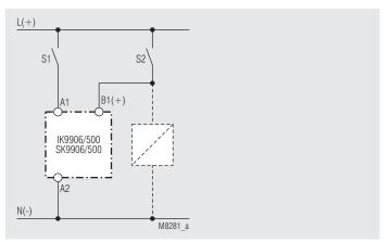
Control with parallel connected load
