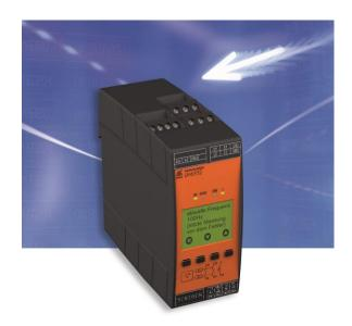
Furthermore, the UH 6932 has a comfortable LCD display and front side buttons, which enable simple operation and rapid configuration of the device without needing a PC. The monitoring function can be deactivated over a digital input or can be activated during operation, with up to four pre-configured speed modes with varying response thresholds. As well as safety-focused contact paths, an analogue output for transfer of the current speed is also available to use.
